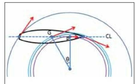
▲ Figure 2: Local drift angle and pivot point
