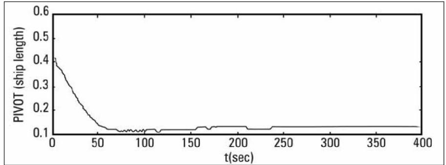
▲ Figure 3: Distance of pivot point from bow, starting from actual point of rotation.
